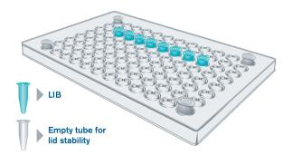
Once the cycler reaches the hybridization temperature during step 2, pause the program, put the HYBs in the thermal cycler, close the lid, and resume the program.
