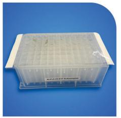
Figure 1: double-sealed plate with "X" cuts
