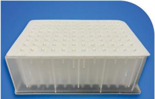
Figure 4: plate fully sealed with silicone mat
